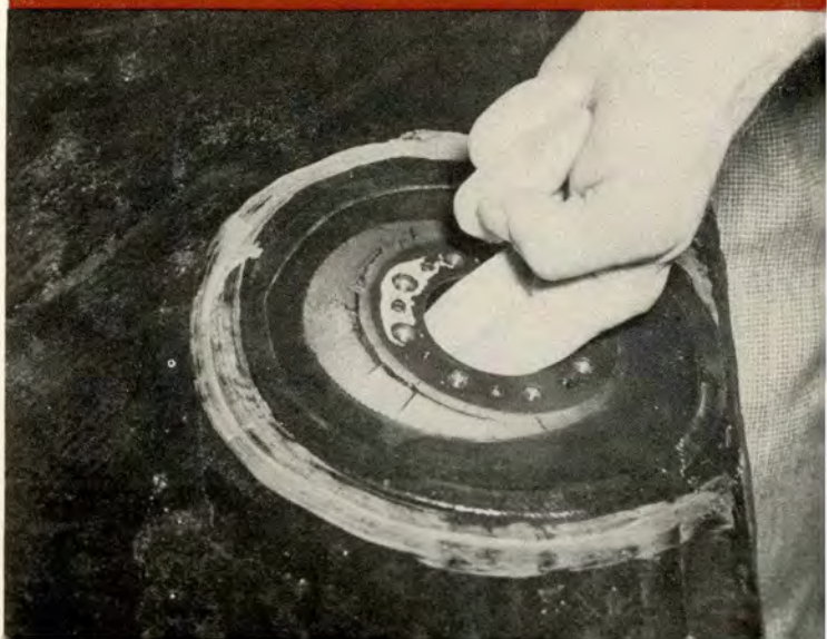
Seals on fuel tank connection parts deteriorated in storage. Crews soon learned where to look for faults.
